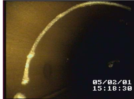
Figure 37 - View of Scrape on the Deposit Surface for Test WAX2001/007 ( \Delta T = 15^\circ\text{F} )
