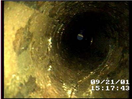
Figure 43 - Deposit on Spool Piece #1 for Test WAX2001/026 ( Q_o=1500 BPD, \Delta T = 15^\circ\text{F} )
