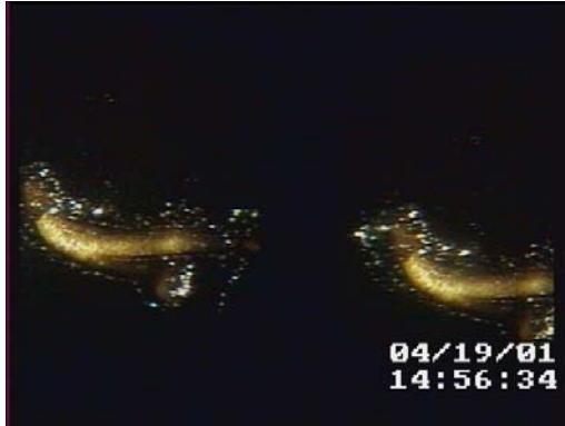
Figure 36 - View of Scrape on the Deposit Surface for Test WAX2001/006 ( \Delta T = 30^\circ\text{F} )
