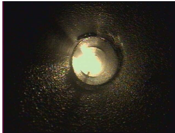
Figure 40 - Deposit on Spool Piece for Test WAX2001/016 ( Q_o = 1800 BPD)
