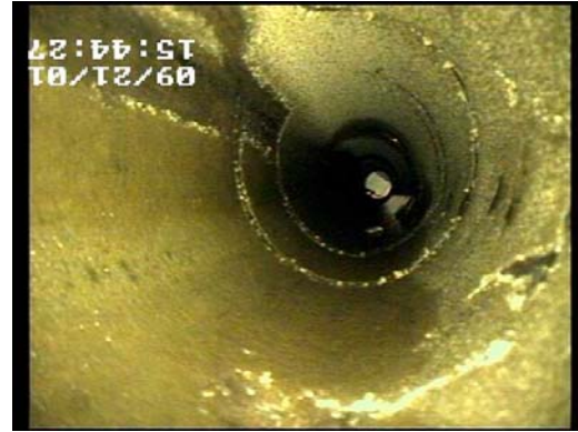
Figure 44 - Deposit on Spool Piece #2 for Test WAX2001/026 ( Q_o=1500 BPD, \Delta T = 15^\circ\text{F} )
