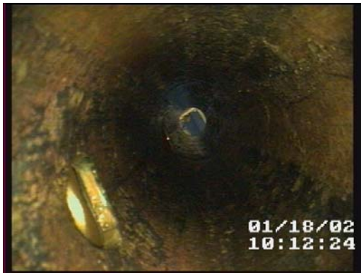
Figure 51 - Deposit on Spool Piece #1 for Test WAX2002/001 ( Q_o = 1800 BPD, \Delta T = 15^\circ\text{F} )
