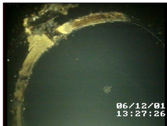
Figure 39 - Deposit on Spool Piece for Test WAX2001/010 (Q o = 2900 BPD)
