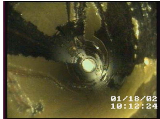
Figure 52 - Deposit on Spool Piece #2 for Test WAX2002/001 ( Q_o = 1800 BPD, \Delta T = 15^\circ\text{F} )
